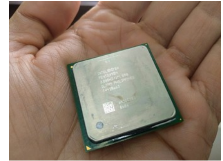
Integrated Circuit Intel Pentium IV (~50Mtt)
