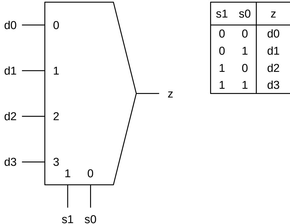
Output z is equal to the data input (dx) selected by the selection inputs (sx)
