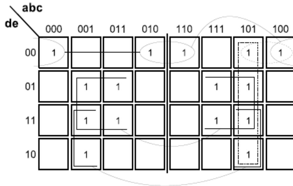
$$f = \bar{c} \bar{d} \bar{e} + ce + \bar{b}cd + a\bar{b}c$$
